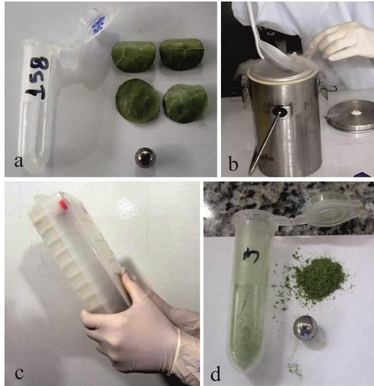
Figure 1. Proposed cacao leaf maceration protocol: a) tube, steel spheres and 15-mm leaf disks; b) freezing the tubes containing the spheres and the leaf discs lyophilized in liquid nitrogen; c) manual agitation of a set of samples; d) fine powder obtained.
